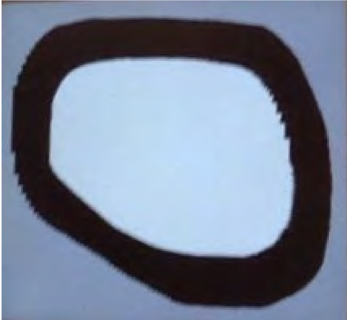
Figure 11: The track regions as processed with our algorithm displayed on a monitor. Grey is the outer track, black is the track, white is the inner track
