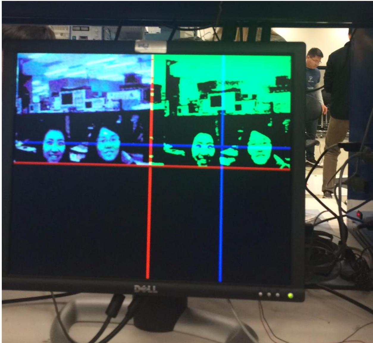
Figure 4: Camera output with 8-bit pixels
