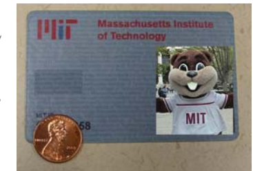
Receiver Powered by 125khz broadcast signal
