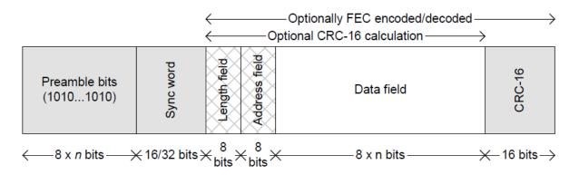
The preamble bits and sync word are used by the receiver for synchronization. For this problem, you will only be concerned with the three blocks of data consisting of the Length Field, Address Field and Data Field. FEC is forward error correction, a technique that allows a receiver to correct errors in a received packet by convolving the data and sending the parity bits. More on FEC in Lpset #7.
