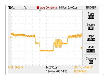
Unlike a PC VGA type display, the NTSC signal is an interlaced signal with 525 scan lines, in two fields of 262.5 lines each. Only 480 lines are visible. Lines 248-263 and 511-525 are blanked on most displays to allow beam to return to the upper left hand corner for the next scan.
