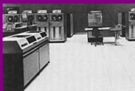
IBM System/360, 1964 500,000 adds/sec
