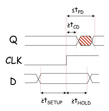
$\textbf{t}_{\text{PD}}\text{:}$  maximum propagation delay, CLK  $\rightarrow Q$
