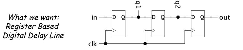
Will nonblocking and blocking assignments both produce the desired result? ("old" means value before clock edge, "new" means the value after most recent assignment)
