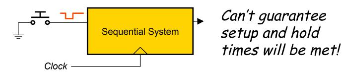
When an asynchronous signal causes a setup/hold violation...
