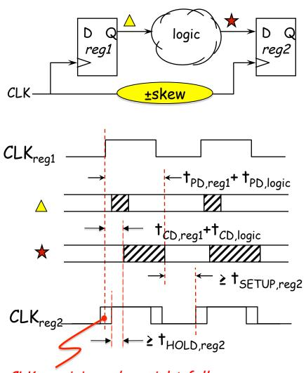
CLK<sub>reg2</sub> rising edge might fall anywhere in this region. In the real world the clock signal arrives at different registers at different times. The difference in arrival times (pos or neg) is called the *clock skew*  $t_{skew}$ .
