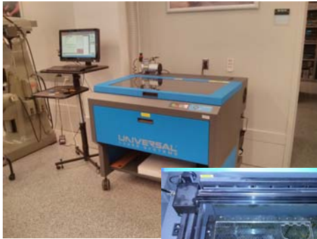
Laser cutter – PSL6.75 with 75W laser Part size: 32" x 18" x 9" Cut by "printing"
