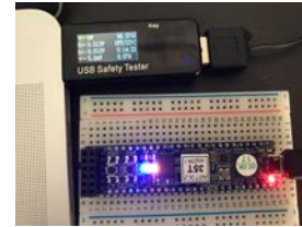
Running Blue LED at 50% duty cycle at 100Hz Based off of 12 MHz clock Consuming 0.35 W
