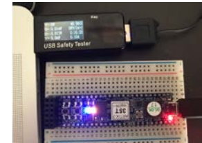
Running Blue LED at 50% duty cycle at 4000Hz Based off of 480 MHz clock Consuming 0.5W
