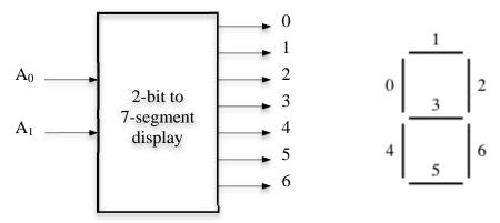
Given the appropriate binary input, this decoder produces outputs that light up the display in the following manner:
