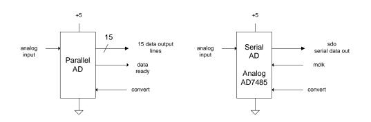
An example of a serial ADC is the Analog Devices AD7485, a 14 bit AD converter with serial output. The AD7485 uses a system clock, MCLK, provided by the user. To start the AD conversion, assert CONVST\_bar (bar = line above CONVST) low. SCO is system clock out which you can ignore for this exercise.
