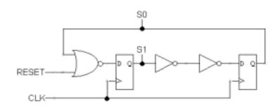
inverter: t<sub>CD</sub>=1ns, t<sub>PD</sub>=2ns nor2: t<sub>CD</sub>=1.5ns, t<sub>PD</sub>=2ns D register: t<sub>CD</sub>=0ns, t<sub>PD</sub>=2ns, t<sub>H</sub>=1ns, t<sub>S</sub>=3ns
