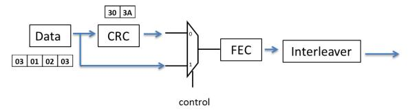
Generating CRC for the four bytes takes 32 clock cycles. Convolution encoding the first four bytes of data also takes 32 clock cycles. Another 16 clock cycle is required to complete the encoding for the CRC for a total of 40 clock cycles. By taking advantage of concurrent processing total processing is reduced from 80 clock cycles to 48 clock cycles.
