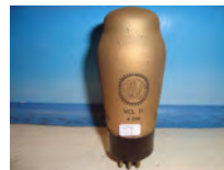
German VCL11, 1938: two tubes in one tube!
