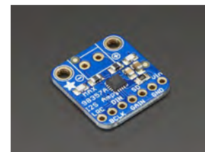
MAX98357A-based board from Adafruit: 3W Class D audio amp i2s input
