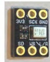
ICS43434 Digital Output Microphone (Invensense), uses i2s protocol
