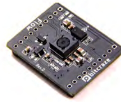
Board with combined PMW3901 and VL53L0X (optical flow and distance)
