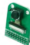
Raw OV2640 (should be able to get 60fps out of this with subsampling)
