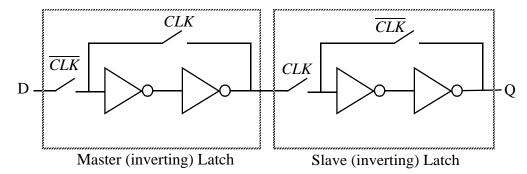
(a) What type of register is shown above (positive edge-triggered or negative edge-triggered)?
