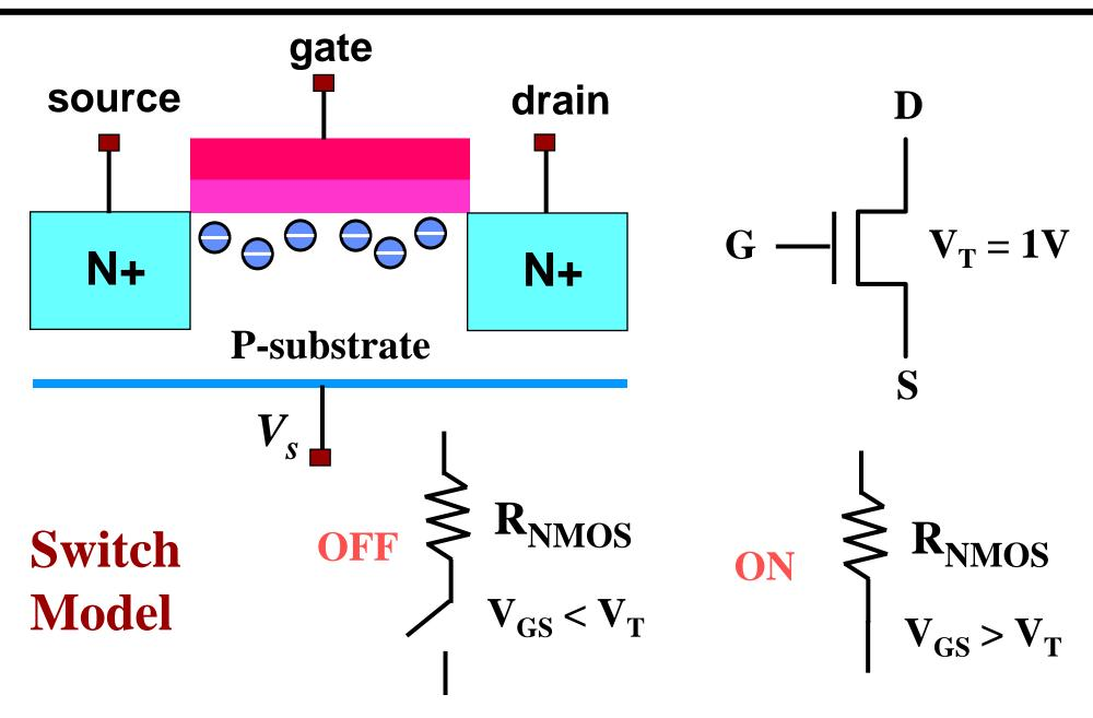
NMOS ON when Switch Input is High
