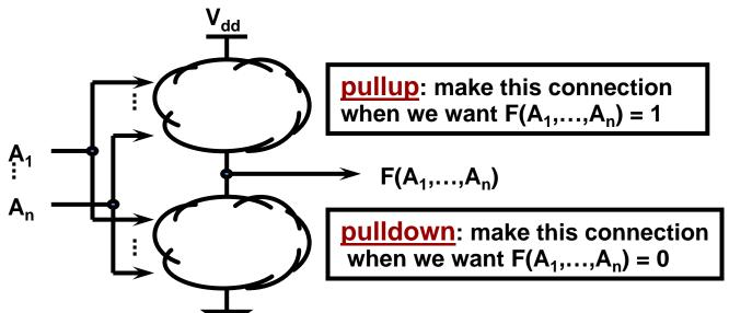
Note: CMOS gates result in inverting functions!
