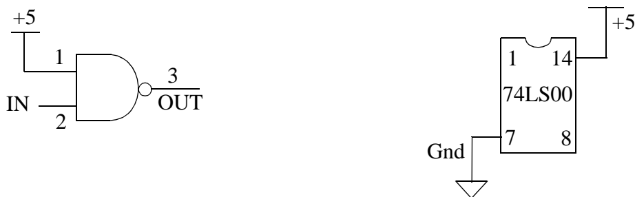
Figure 1: (a) Logic Level Measurement (Measure voltage at OUT node). (b) Power Supply Wiring.
