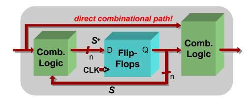
Since outputs are determined by state and inputs, Mealy FSMs may need fewer states than Moore FSM implementations
