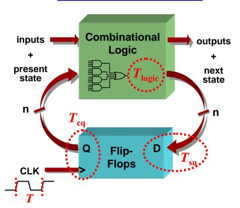
$$T > T_{cq} + T_{logic} + T_{su}$$
