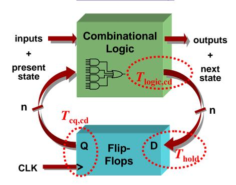
$$T_{cq,cd} + T_{logic,cd} > T_{hold}$$
