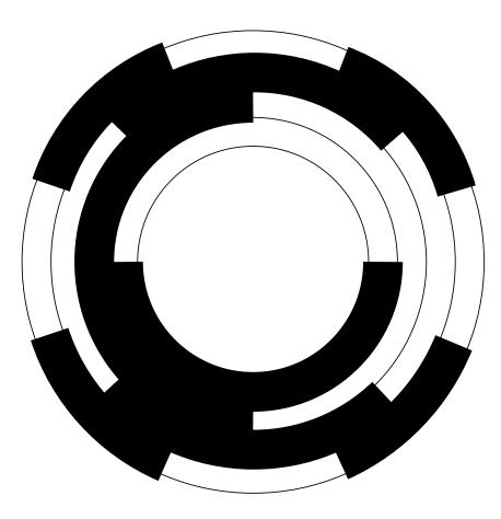
Here is a 4–bit (22.5 degree) resolution wheel. 0 0 **One source per sensor** 0 0 0 0 1 bit. 0 0 1 1 1 0 Can make these wider. 0 1 1 **Resolution is** 0 1 0 1 1 0 0 **360**<sup>0</sup> 1 0  $2^{\overline{N}}$ 1 1 1 1 Use a Gray code to 1 eliminate chatter. 0 1 1
