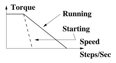
Must sometimes 'ramp up' speed. Holding torque is limited by heating and by saturation.
