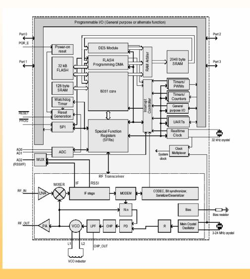
CC1010 (ChipCon) -8051 Compatible Microcontroller -300-1000 MHz RF Transmission -32 kB Flash Memory -A/D Converter (10 bit)
