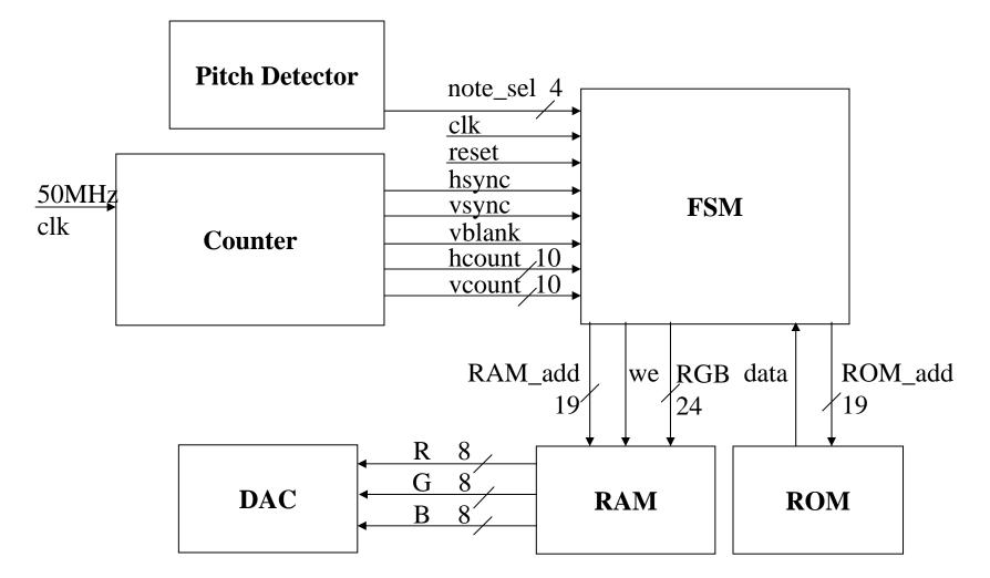
FSM contains minor FSMs which are controlled by a major FSM800 x 600 display, 72Hz
