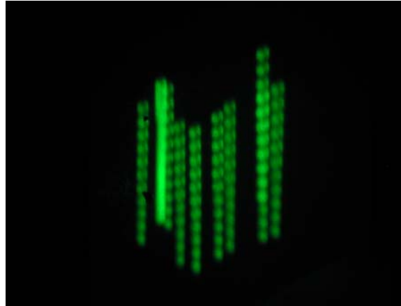
Figure 19: The projected laser raster test pattern prior to mirror alignment.
