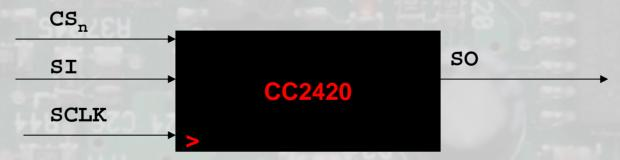
•All operations performed by writing or reading from 33 16-bit configuration registers and 15 8-bit command strobe registers
