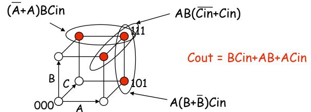
The on-set is completely covered by the combination (OR) of the subcubes of lower dimensionality - note that "111" is covered three times
