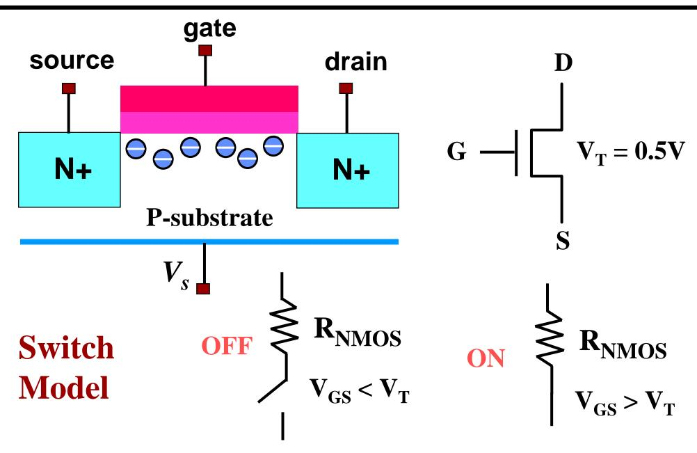
NMOS ON when Switch Input is High
