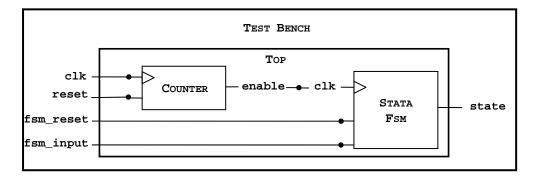
First create a file called top.v, in which you instantiate the counter module from Problem 1 and the **Stata\_FSM** module from Problem 2. Next create a file called **testbench.v**, in which you instantiate the top module and specify the timescale as below such that time units are in nanoseconds.
