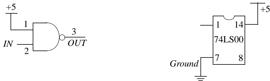
Figure 1: (a) Logic Level Measurement (Measure voltage at OUT node). (b) Power Supply Wiring.
