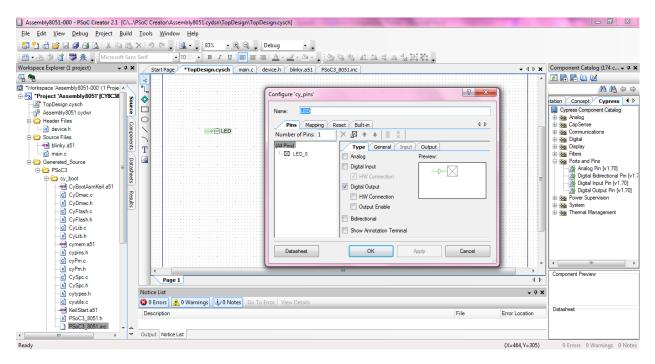
By linking this internal pin to a physical pin on the chip, we can send our PWM signal to the pin attached to the LED on the kit. We can vary the duty cycle of this blinking as usual—by changing the values of the registers R0-R2 in the above code.
