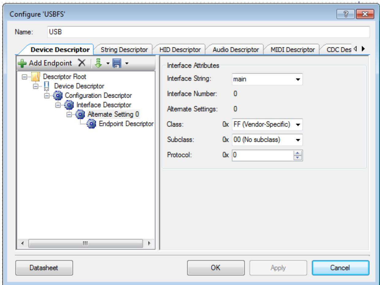
Here comes the point where we actually decide how we are going to communicate. Endpoints are unidirectional (except for control transfers) communication channels that can be designated to specific tasks by the driver. In this case we need two endpoints, one for in (into the Host or out from the PSoC), and one for out (out from the Host or into the PSoC), so press the “Add Endpoint” button. Select the first endpoint and set the settings as follows:
