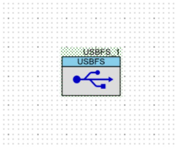
Open the configuration screen by double clicking the component. Change its name to USB. Under ‘Descriptor Root’, highlight the ‘Device Descriptor’ label and set the values as follows:
