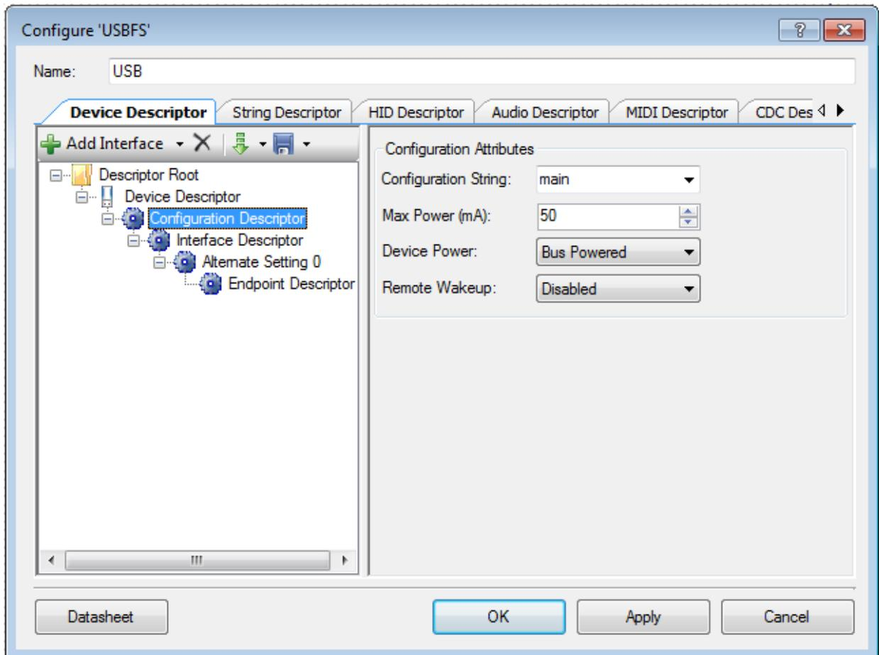
Onto 'Alternate Setting 0'. Set the values as shown below:
