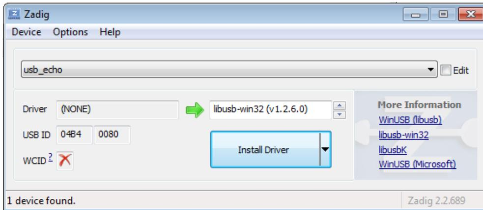
Once the driver is installed, in the windows Device Manager (can be search for in the Start Menu), your device should show up under 'libusb-win32 device' if it installed correctly
