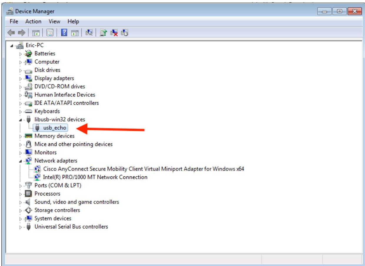
Now that this device has been successfully installed, we need to install PyUSB. Fortunately, Python comes with a package manager called pip. To install pyusb simply enter the command ``pip install pyusb`` into your command line.
