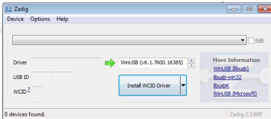
Then, plug in your device through the USB port (generally not the same port used to program the device) and it should show up in Zadig. Set the driver type to libusb-win32 and press install.
