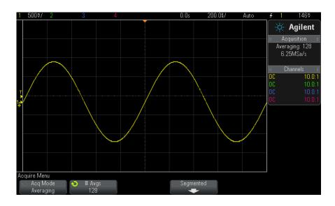
Figure 39 128 Averages used to reduce random noise
