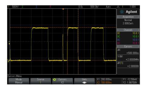
Figure 43 Measuring pulse width with cursors
