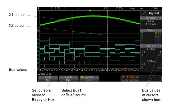
Bus values are displayed when using Pattern trigger The bus values are also displayed when using the Pattern trigger function. Press the **[Pattern]** key on the front panel to display the Pattern Trigger Menu and the bus values will be displayed on the right, above the softkeys.
