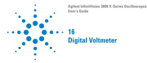
The Digital Voltmeter (DVM) analysis feature provides 3-digit voltage and 5-digit frequency measurements using any analog channel. DVM measurements are asynchronous from the oscilloscope's acquisition system and are always acquiring.
