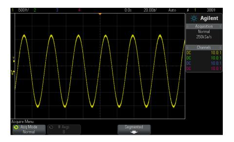
Figure 36 Sine With Glitch, Normal Mode
