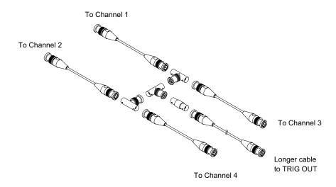
Figure 50 User Calibration cable for 4-channel oscilloscope
