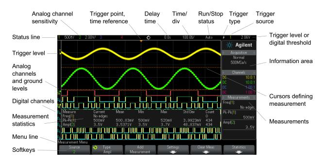
Figure 1 Interpreting the oscilloscope display
