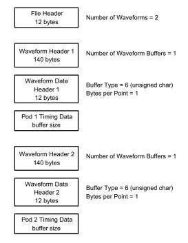
Segmented Memory Acquisition on One Analog Channel The following picture shows a binary file of a segmented memory acquisition on one analog channel.
