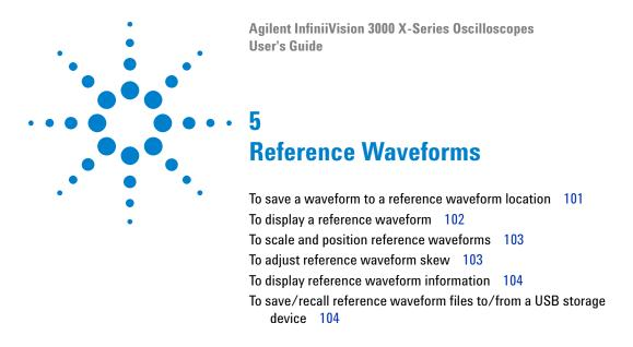
Analog channel or math waveforms can be saved to one of two reference waveform locations in the oscilloscope. Then, a reference waveform can be displayed and compared against other waveforms. One reference waveform can be displayed at a time.
