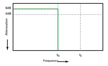
Figure 34 Theoretical Brick-Wall Frequency Response
