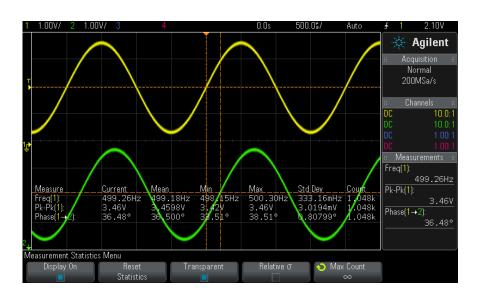
The following statistics are shown: Name of the measurement, current measured value, mean, minimum measured value, maximum measured value, standard deviation, and the number of times the measurement has been made (count). Statistics are based on the total number of captured waveforms (count).
