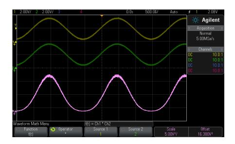
Figure 6 Example of Multiply Channel 1 by Channel 2
