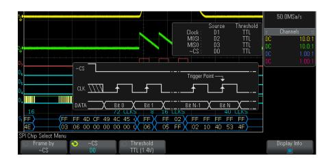
**9** Press the **CS** softkey to open the SPI Chip Select Menu.
