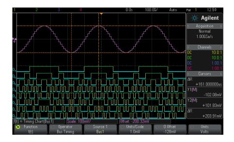
Figure 18 Example of Chart Logic Bus Timing
