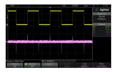
Figure 7 Example of Differentiate Function
