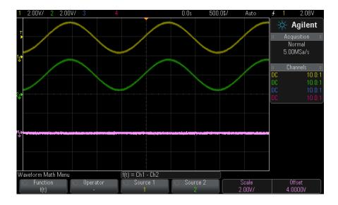
Figure 5 Example of Subtract Channel 2 from Channel 1
