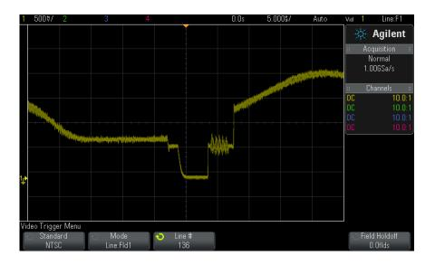
Figure 27 Example: Triggering on Line 136
