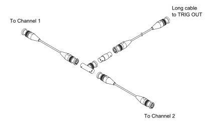
Figure 49 User Calibration cable for 2-channel oscilloscope
