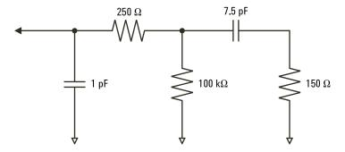
Figure 22 High-Frequency Probe Equivalent Circuit
