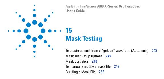
One way to verify a waveform's compliance to a particular set of parameters is to use mask testing. A mask defines a region of the oscilloscope's display in which the waveform must remain in order to comply with chosen parameters. Compliance to the mask is verified point-by-point across the display. Mask test operates on displayed analog channels; it does not operate on channels that are not displayed.
