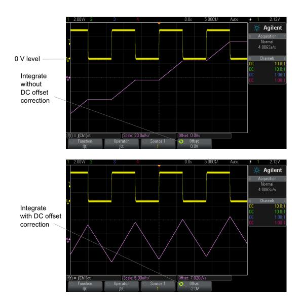
Figure 8 Integrate and Signal Offset
