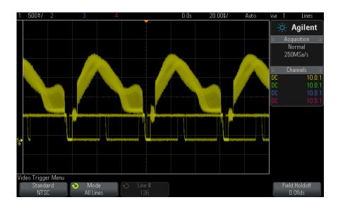
Figure 28 Triggering on All Lines
