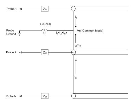
Figure 24 Common Mode Input Voltage Model
