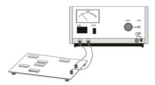
**2** Connect the digital probe cable to the DIGITAL Dn - D0 connector on the front panel of the mixed-signal oscilloscope. The digital probe cable is keyed so you can connect it only one way. You do not need to power-off the oscilloscope.
