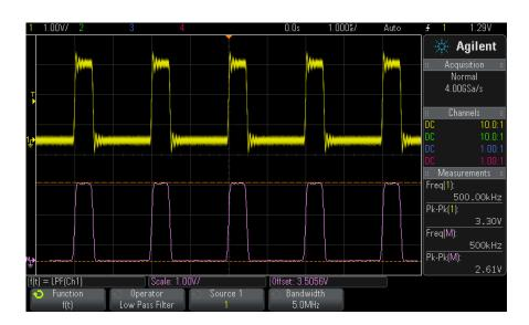
Figure 15 Example of Low Pass Filter
