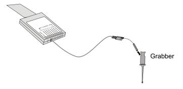
5 Connect the grabber to a node in the circuit you want to test.
