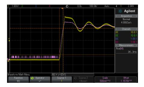
**Figure 10** Example of  $\sqrt{\text{(Square Root)}}$
