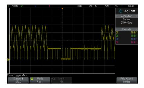
Figure 29 Triggering on Field 1
