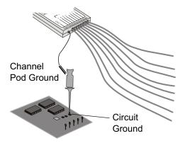
**4** Connect a grabber to one of the probe leads. (Other probe leads are omitted from the figure for clarity.)
