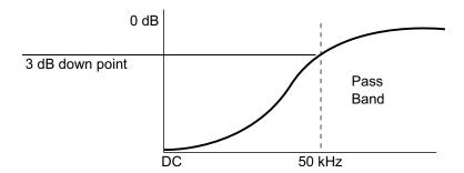
Low frequency reject removes any unwanted low frequency components from a trigger waveform, such as power line frequencies, etc., that can interfere with proper triggering.
