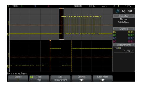
Figure 48 Isolating an event for Frequency measurement
