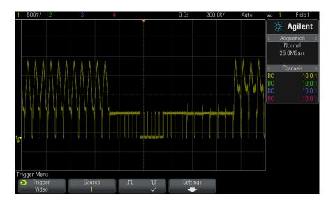
**3** Press the **Source** softkey and select any analog channel as the video trigger source.
