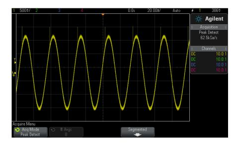
Figure 37 Sine With Glitch, Peak Detect Mode
