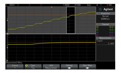
Figure 46 Isolating area for Top measurement
