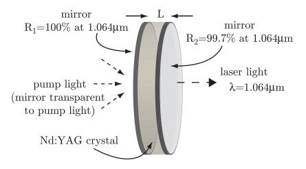
Assume the lower and upper laser levels ( $E_1$  and  $E_2$  respectively) have an energy separation corresponding to  $\lambda = 1.064 \ \mu m$ .
