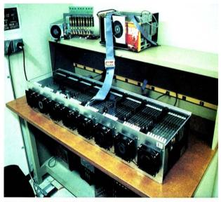
The nodes are packaged as one circuit board per node in the long card frame on the bench top. The six communication channels from each node are wired in a binary 6-cube on the backplane on the underside of the card frame. The separate
