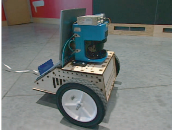
Figure 7: Splinter. This is the robot that collected the dataset. The vehicle, known as “Splinter”, has high quality quadrature phase encoders on each drive motor. A laptop on the back of the vehicle logged the data. The large blue device in the front of the vehicle is a laser range finder, not used in this article.
