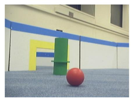
This image, capture3.png, is a sample from a playing field. We will use it to see how to read data from disk, search it for red blobs, draw on it, and write the modified image back to disk. In particular, we will scan for red pixels, compute some statistics about them (area, center of mass, bounding box, aspect ratio), draw the bounding box, draw an X at the center of mass, and color in all the pixels we thought were red.
