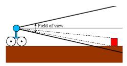
Depending on how well you can find red balls, you might be able to use the size of the ball as an indicator of validity and distance. If you have a ball that has an area of only two pixels, it's a good bet that it's either noise, or only part of a ball. Depending on the orientation of your camera, you may also be able to tell if a red blob you found is floating in mid-air.
