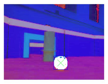
Why are the colors so weird? Well, we converted the image to the HSV color space, storing the hue in the red channel, the saturation in the green channel, and the value in the blue channel. That's why the walls look blue—very large value, whereas (what you can see of) the ball looks red—very large hue.
