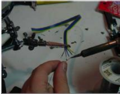
Pre-tin (add some solder) the stranded wire.
