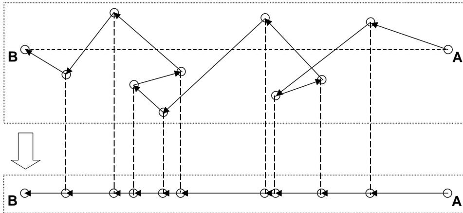
Figure 3: Every non-collinear network with links that have negative projections along  $AB$  can be transformed into a more efficient collinear network with links only in the  $AB$  direction.
