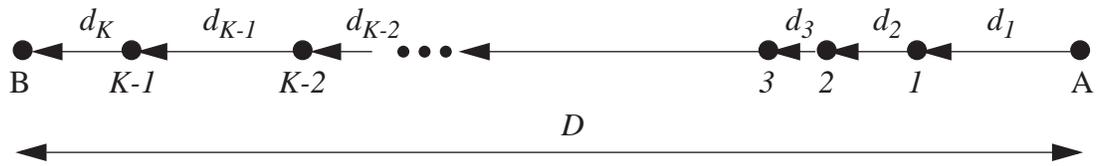
Figure 2: Introducing  $K - 1$  relay nodes between  $A$  and  $B$  to reduce energy needed to transmit a bit.
