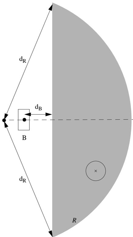
Figure 13: Gathering data from a source that resides in a sector (subtending angle  $2\theta$  at the centre)  $d_B$  away from the basestation ( $B$ ).
