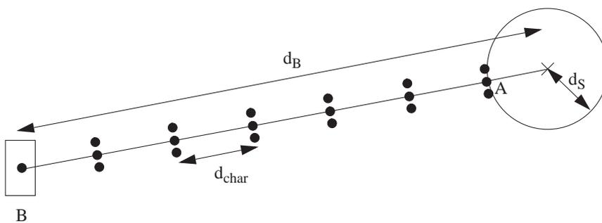
Figure 6: An example network that achieves the upper bound on lifetime. Here,  $d_B - d_S = 6d_{char}$  i.e.  $M = 6$  and  $N = 18 = 3(6)$  i.e.  $P = 3$ . Thus there are 3 parallel minimum-energy backbones of 6 nodes each.
