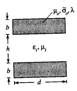
Two identical, thick  $(\lambda \ll b)$  superconducting plates.
