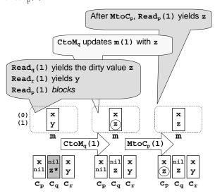
Here are the possible transitions of IncoherentMemory for a given address. This kind of state transition picture is the standard way to describe cache algorithms in the literature; see pages 664-5 of Hennessy and Patterson, for example.
