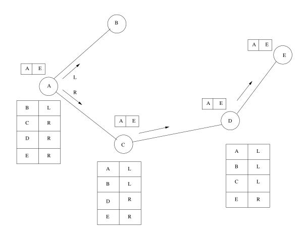
An example of data routing in Internet using routing table informtion Q: How to configure these routing tables?
