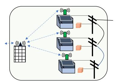
Figure 2: A microgrid. Each house has solar panels, batteries, and a smart meter. It is connected to the power lines, which form a local loop with a connection to the central power utility. A microgrid controller controls it and communicate with LTE to both the individual smart meters and the central utility
