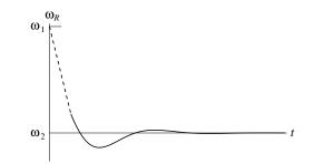
4. Assuming the model represented by the sketch above is correct, how much kinetic energy was contained in the oscillatory motion of the washer with respect to the rotor at the time when  $\omega_R = \omega_{R\min}$ ?
