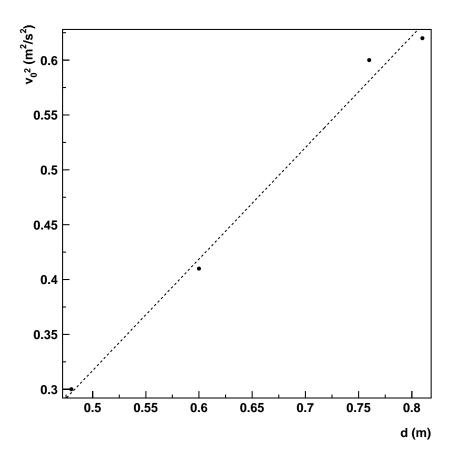
The slope, calculated using a computer program, is 1.02 m/s<sup>2</sup>. So the coefficient of friction is  $\mu_k$ =slope/2g=0.05.
