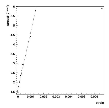
From the slope in the linear regime, the Young's modulus of this wire is  $3 \times 10^{10} \text{ N/m}^2$ . The tensile strength of the wire is roughly the stress at the breaking point, or  $1.3 \times 10^8 \text{ N/m}^2$ .
