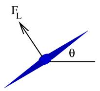
The pressure of the air against the bottom of the airplane's wings exerts a "lift" force  $F_L$ . The direction of this force is always perpendicular to the wings. The airplane has mass M. The airplane's engines exert a forward "thrust" force on the plane  $F_t$ , while air resistance exerts a backward "drag" force  $F_d$ . ("Forwards" and "backwards" mean with respect to the direction of motion of the airplane.)
