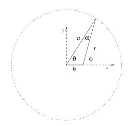
where the angles and the distance r are defined by the figure. Note that r is not the radius of the circle, but the distance from the current element  $dI = K a d\theta$  to the point on the x-axis where we want to find the field. Note also that for  $\theta$  and hence  $\phi$  in the first quadrant,  $dB_y$  is negative, as expected. Note even further that I can't get the graphics program to give me  $\phi$  in the font I want.
