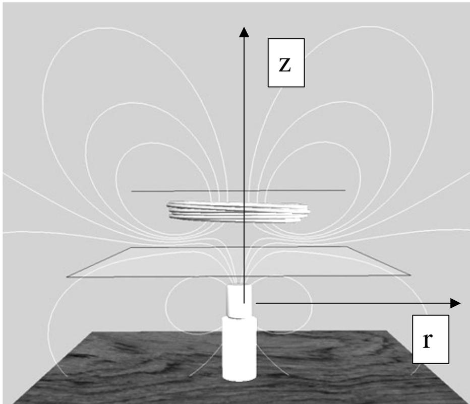
(a) Using a battery attached to the coil, you run a current  $I$  in the coil. Viewed from above, in what direction do you want the current in the coil to flow (clockwise or counterclockwise) so that the  $d\vec{F} = Id\vec{l} \times \vec{B}$  force has an upward component?
