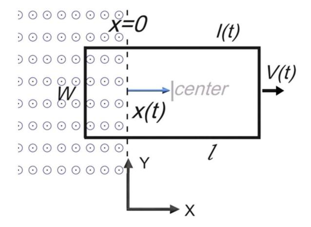
A rectangular loop lies in the xy plane and is made out of wire with zero resistance. The loop has mass m, inductance L, width W, and length I. It oscillates back and forth with frequency  $\omega$  in the x-direction in an external magnetic field that is out of the page for x < 0 with magnitude  $B_o$ , and zero for x > 0. There are no frictional or gravitational forces in this problem. The position x(t) of the center of the loop at time t is given by
