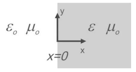
A electromagnetic plane wave propagating from the left is incident on a dielectric with dielectric constant  $K_e$ . The incident electric field is polarized in the y direction. The dielectric occupies all space for x > 0. For x < 0 we have vacuum. Our electric and magnetic fields are given by
