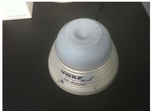
FIG. 19. Image of Vortexer used to vibrate the solution.
