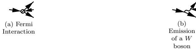
FIG. 3: Feynman diagrams of the muon decay process, in which the time axis is directed to the right. Figure (a) represents Fermi’s original theory of interaction, while figure (b) reflects a modern understanding of the electroweak interaction. Note an arrow to the right indicates a particle travelling forward in time, while an arrow to the left indicates an antiparticle travelling forward in time.
