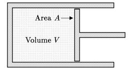
Let U denote the total energy of the gas, and let p denote the pressure. Suppose that the piston is moved a distance dx to the right. (We suppose that the motion is slow, so that the gas particles have time to respond and to maintain a uniform pressure throughout the volume.) The gas exerts a force pA on the piston, so the gas does work dW = pAdx as the piston is moved. Note that the volume increases by an amount dV = Adx, so dW = pdV. The energy of the gas decreases by this amount, so
