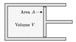
Let U denote the total energy of the gas, and let p denote the pressure. Suppose that the piston is moved a distance dx to the right. (We suppose that the motion is slow, so that the gas particles have time to respond and to maintain a uniform pressure throughout the volume.) The gas exerts a force pA on the piston, so the gas does work dW = pAdx as the piston is moved. Note that the volume increases by an amount dV = Adx, so dW = pdV. The energy of the gas decreases by this amount, so
