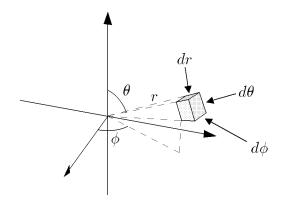
The cell includes the volume lying between r and r + dr, between  $\theta$  and  $\theta + d\theta$ , and between  $\phi$  and  $\phi + d\phi$ . In the limit as dr,  $d\theta$ , and  $d\phi$  all approach zero, the cell approaches a rectangular solid with sides of length:
