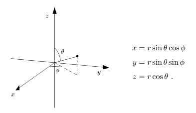
The equator is then described by  $\theta = \pi/2$ , and  $\phi = \psi$ , where  $\psi$  is a parameter running from 0 to  $2\pi$ . Thus, the equator is described by the curve  $x^i(\psi)$ , where
