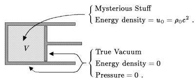
The piston is then pulled outward, so that its initial volume V is increased to  $V + \Delta V$ . You may consider  $\Delta V$  to be infinitesimal, so  $\Delta V^2$  can be neglected.
